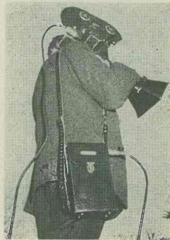
The electrical requirements for this ciné camera are met by the DEAC battery in the leather case. (See 'Rechargeable Batteries').
