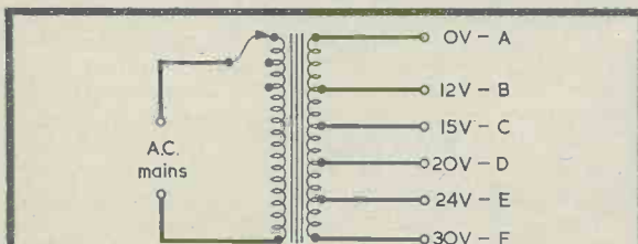
Fig. 1. The secondary voltages offered by the Douglas mains transformer Type MT3
